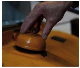
Air intake valve on Ossberger Crossflow
